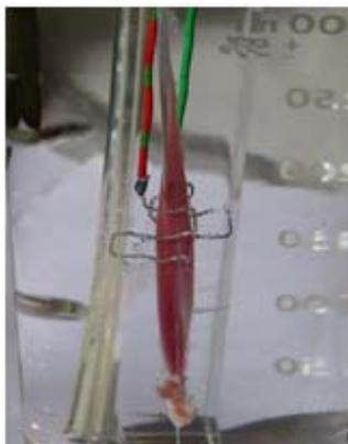
**Figure 5:** M. extensor digitorum lateralis mounted vertically inside the experimental chamber. The proximal tendon is facing the bottom of the glass. Muscle is surrounded by bubbled Krebs - Henseleit Buffer and flanking horizontally both platinum electrodes.
