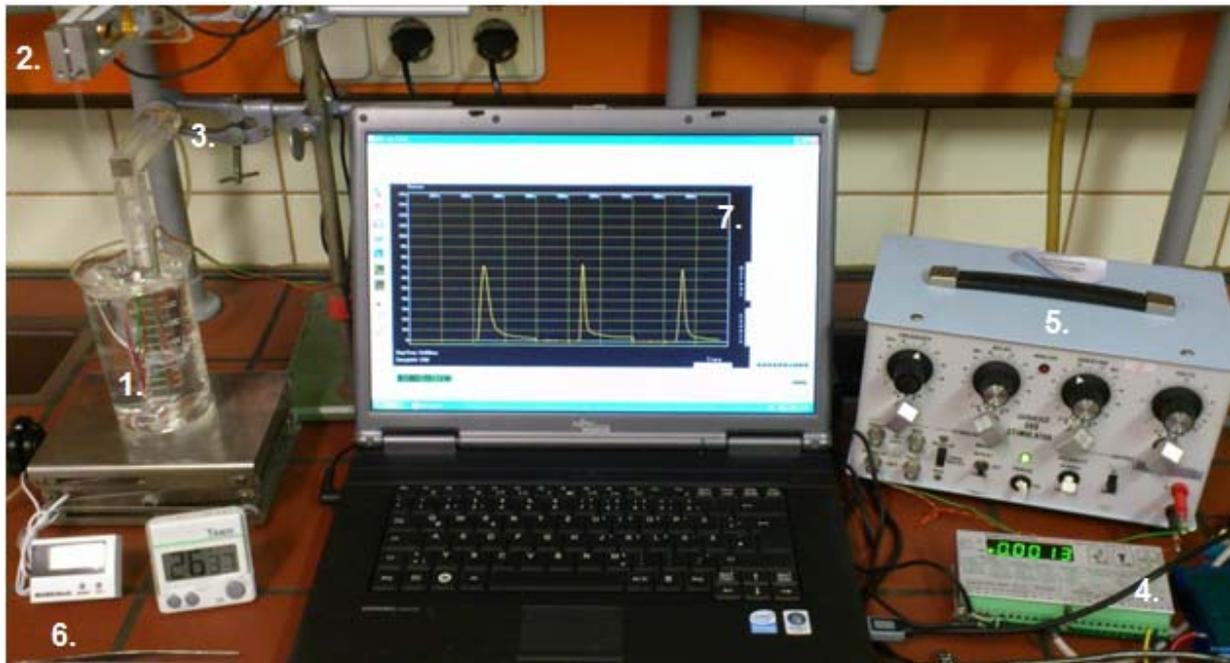
**Figure 7:** Overview of all system components. 1. Muscle containing chamber, 2. Isometric & isotonic force transducer, 3. Muscle holder, 4. Signal enhancer, 5. Pulse generator, 6. Thermometer, 7. Software.
