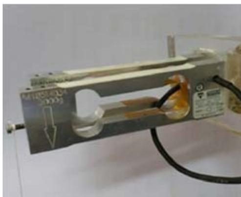
**Figure 6:** Both force transducers connected to a Plexiglas. Front transducer is immobilized and hence used for isometric measurements. The other transducer was moveable and therefore used for isotonic measurements.
